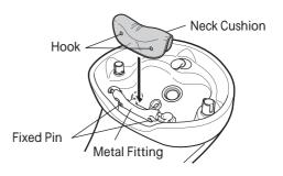
2. Both side hooks of the neck cushion is xed on a xed pin.
